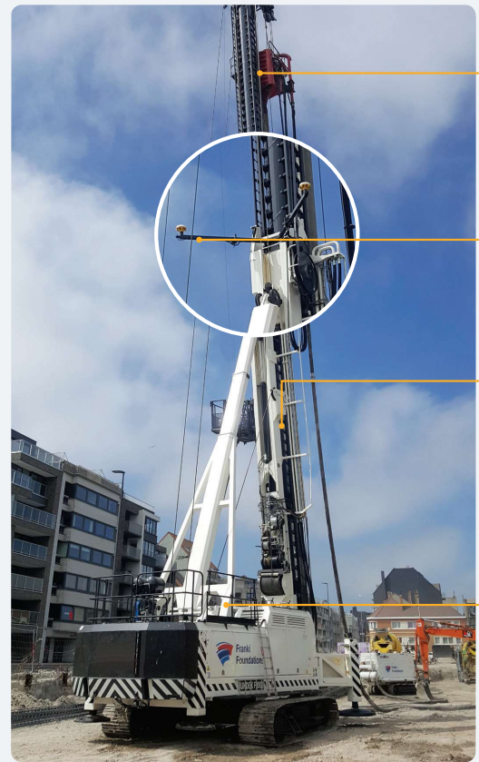
Trimble Display, GNSS Receiver, CAN to Ethernet Adapter, Ethernet Switch, Power Conditioner (Optional) Modem for cellular or Wi-Fi connectivity
