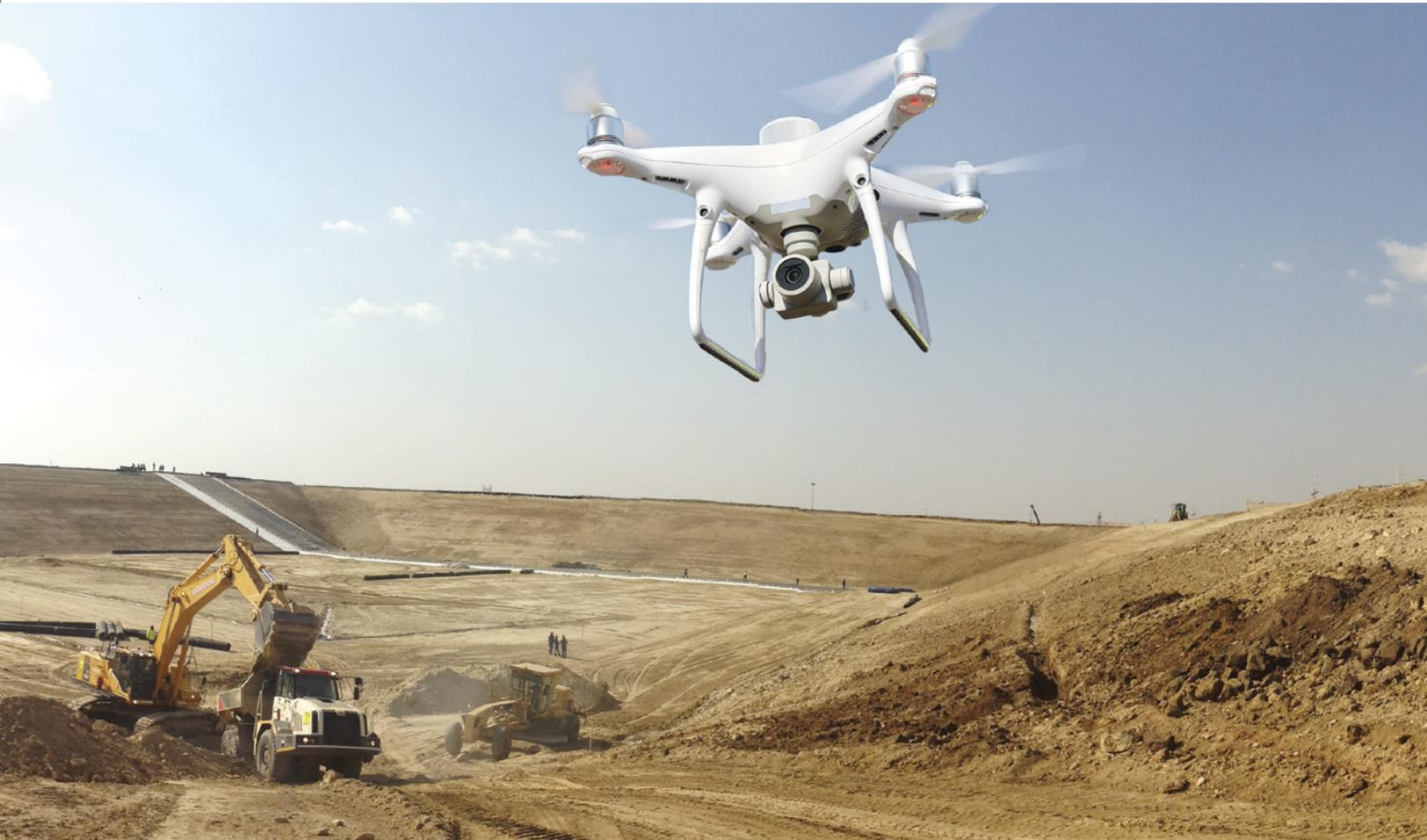
The GNSS data files are post processed, and time stamps (event markers) are used to accurately geotag the images.
