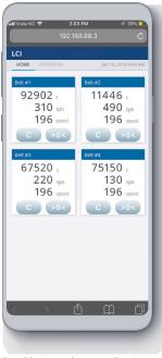
The LCI collects real time data from your Loadrite belt scales networked for display in the control room.
