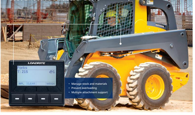
Cost-effective, compact, all-weather measurement of construction materials and farm feeds. The Loadrite<sup>®</sup> S1100 is an on board scale that helps the operator to accurately weigh every lift, track loading totals, prevent overloading and effectively manage stock. So you can improve safety and profitability through increased efficiency and accuracy.
